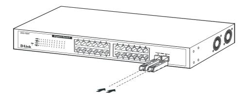
Figure 1- 5. Mini-GBIC modules plug-in to the Switch
